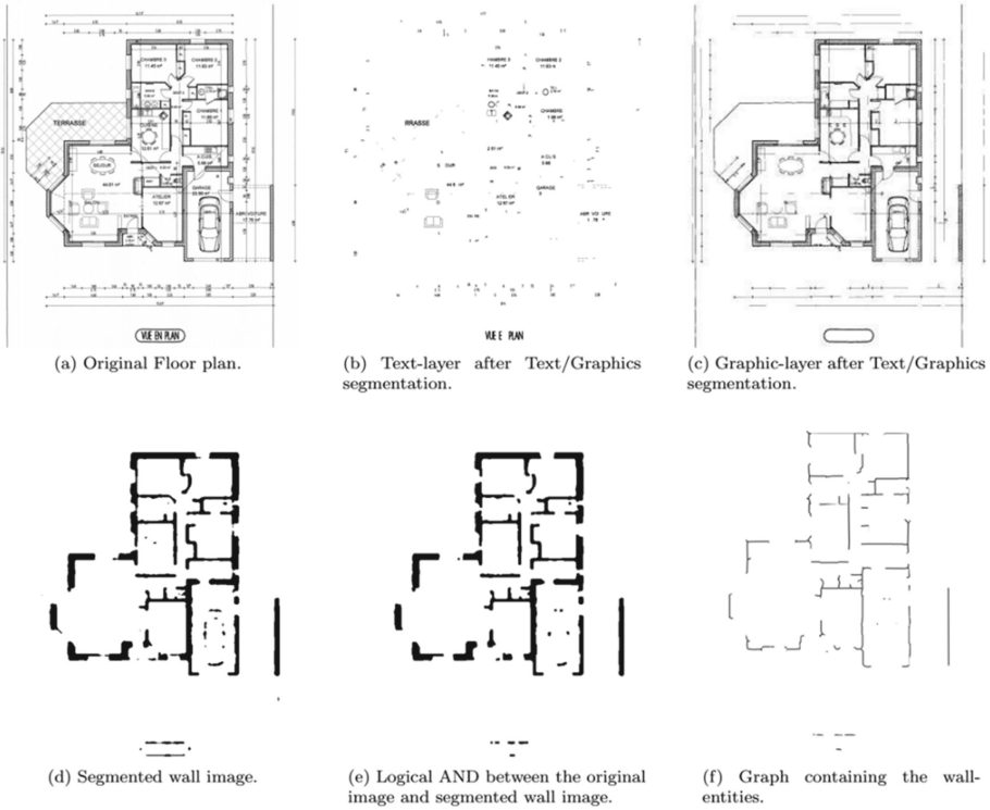
Fig. 1. Complete flow of wall recognition process in [3] (Image from [3]).
